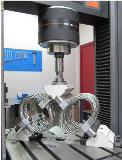
Figure 3 – Characterisation test on isolators
