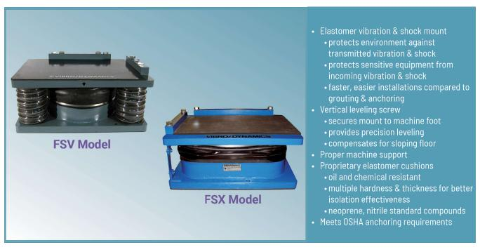
FSV<sup>™</sup> and FSX<sup>™</sup> Spring Mounts provide the ultimate in shock isolation effectiveness. Their low stiffness and natural frequency results in shock isolation in the 80-90 percent range. Hammer motion is controlled by a very sophisticated viscous damper design, providing a fast decay of motion between hammer blows.
