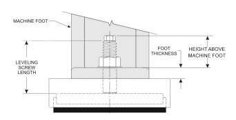
The Chart below is used to determine the the height of a Leveling Adjustment Screw above the Isolator Housing.
