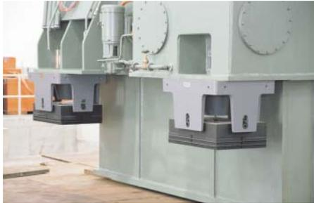
The isolators are attached to the press feet.
