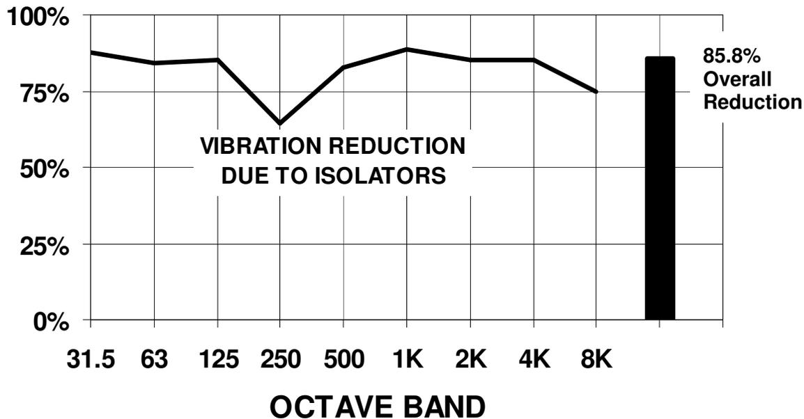
EFFECTIVENESS OF SERIES BFM 1230 MICRO/LEVEL ISOLATORS IN REDUCING VIBRATION CAUSED BY A 250 TON BLANKING PRESS
