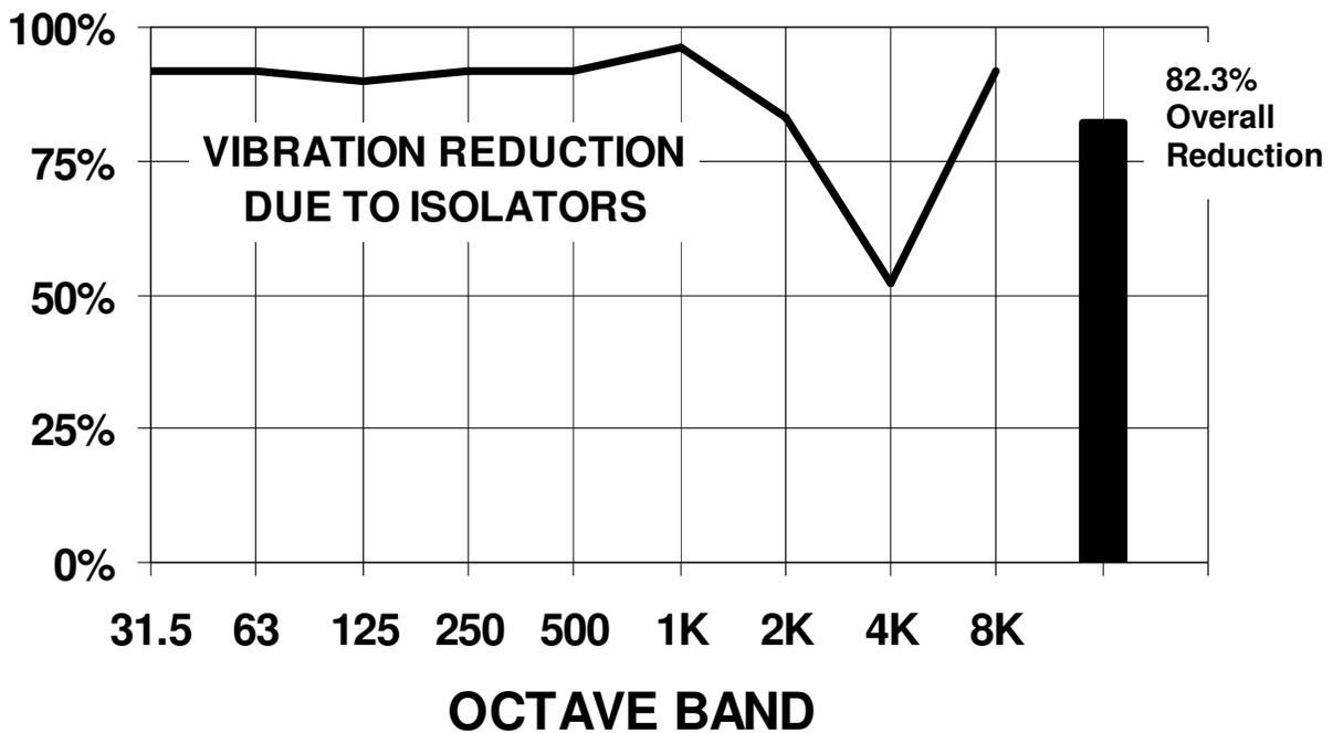
EFFECTIVENESS OF SERIES BFM 1230 MICRO/LEVEL ISOLATORS IN REDUCING VIBRATION CAUSED BY A 250 TON BLANKING PRESS
