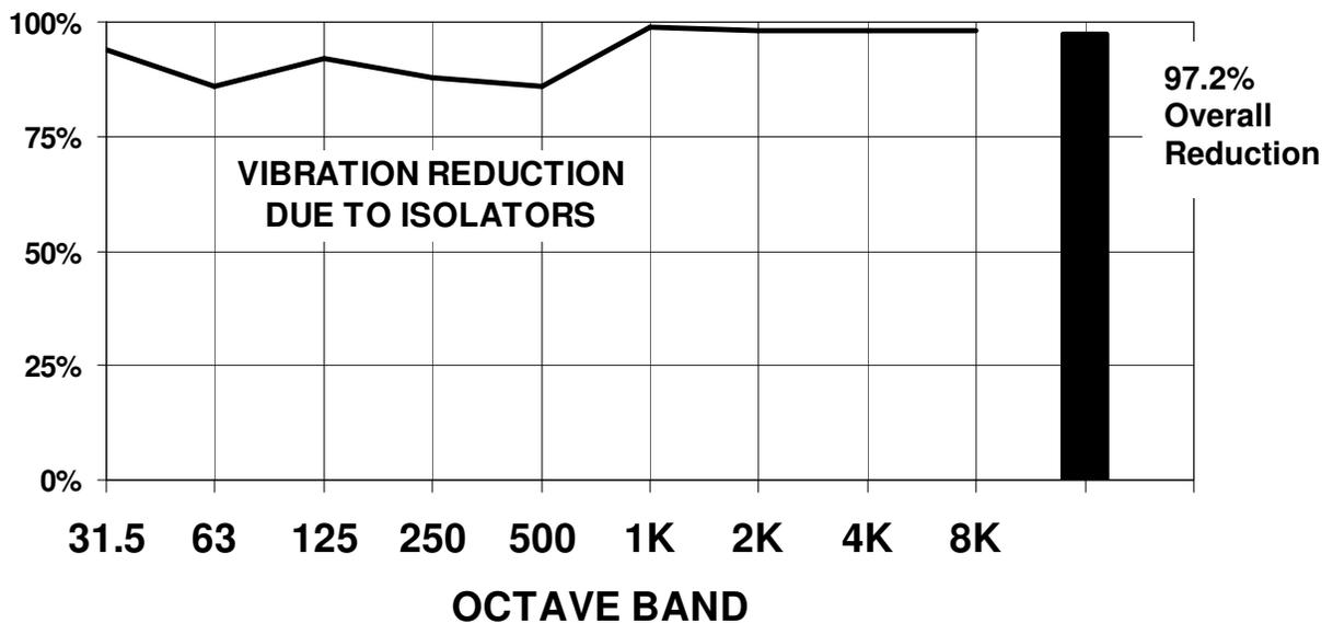
EFFECTIVENESS OF SERIES BFM 1230 MICRO/LEVEL ISOLATORS IN REDUCING VIBRATION CAUSED BY A 250 TON BLANKING PRESS
